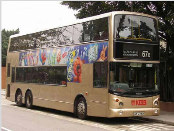
Trident launched Super Low Floor entry EuroII emissions engine
