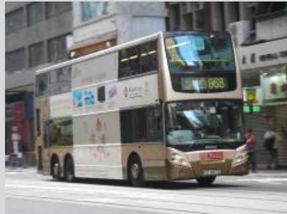
Enviro500 Next Generation Lighter weight Increased seating capacity ZF axles – disc brakes all round Major focus on all-round improvements Euro5 emissions engine ZF Ecolife transmission
