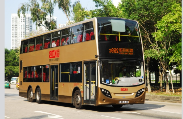
Enviro500 Next Generation Lighter weight Increased seating capacity ZF axles – disc brakes all round Major focus on all-round improvements Euro5 emissions engine ZF Ecolife transmission
