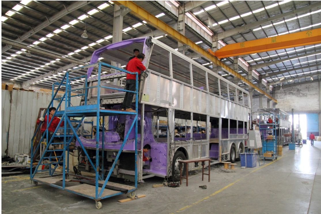
The bus formed its shape with body components integrated together and attached on the chassis (Benny Sit)
