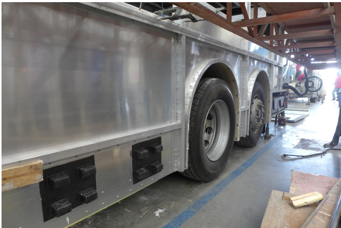
Close-up of aluminium-made nearside body frame (Edmund Leung)
